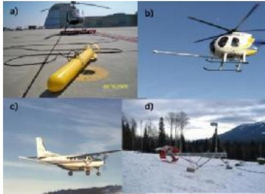
Figure 1.1 Various airborne magnetometers. Photo a) shows a helicopter-towed bird sensor. Photo b) shows a sensor mounted on a nose stinger on a helicopter. Photo c) shows a tail stinger mounted sensor. Photo d) shows a gradiometer bird for helicopter surveys.
