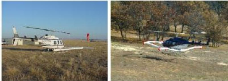
Figure 1.11 Helicopter deployed magnetometer arrays. On the left is shown a single sensor array from Sky Research. On the right a gradiometer array from Battelle is shown.
