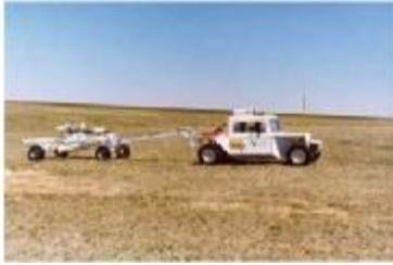
Figure 1.10 Land-based magnetometer array known as Multi-Sensor Towed Array Detection System (MTADS)
