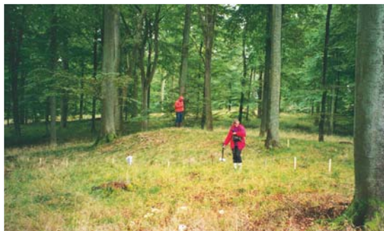
Glarborg, Zealand, Denmark. 2001. Above: Scheme of magnetic survey with one gradiometer GSM-19 (one sensor is on the base point to control temporal variations; it is connected to the console with a 50 m long cable). Graphs of the measured magnetic field are shown. Below: At work with the magnetic survey. One operator is collecting magnetic data, the other one is measuring GPS coordinates of the plot.
