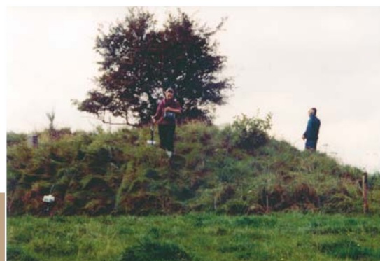
Glarborg, Zealand, Denmark. 2001. Above: Scheme of magnetic survey with one gradiometer GSM-19 (one sensor is on the base point to control temporal variations; it is connected to the console with a 50 m long cable). Graphs of the measured magnetic field are shown. Below: At work with the magnetic survey. One operator is collecting magnetic data, the other one is measuring GPS coordinates of the plot.
