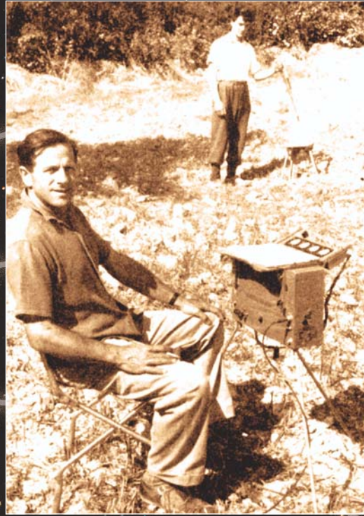
Martin Aitken using the prototype proton magnetometer. The detector bottle is supported on a tripod in the background. (Adapted after Clark, 1990, p. 17).
