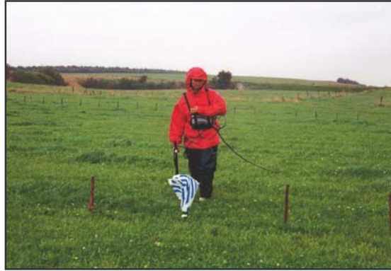
Hov, Thy. Magnetic surveying on the western part of the site. The reference sensor is covered with a plastic pack against rain. 2002.
