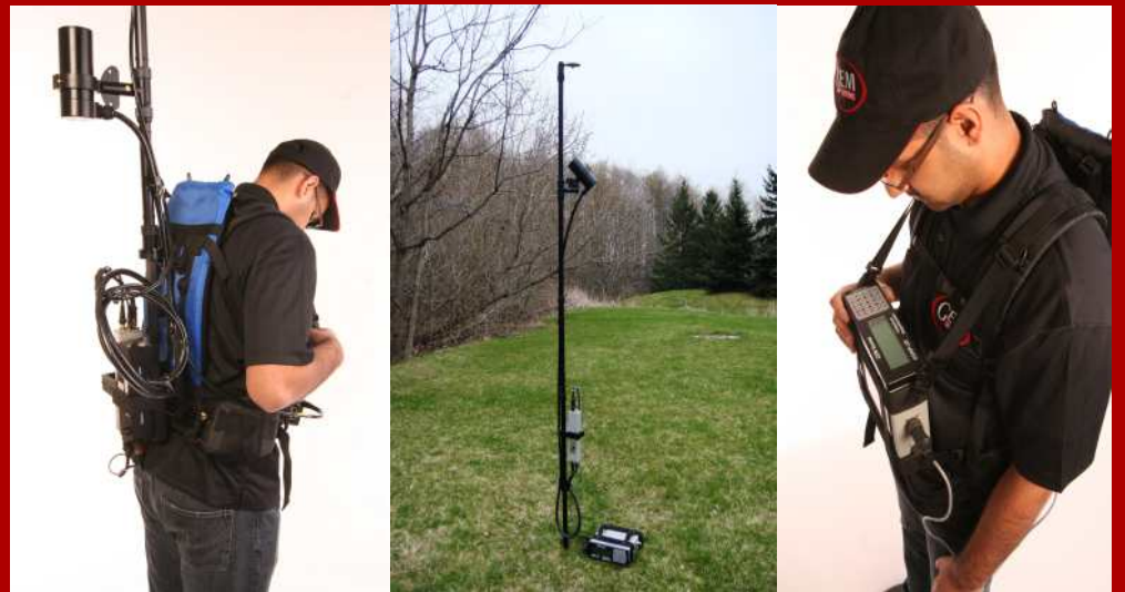
Optically pumped Potassium Magnetometer with ruggedized console, backpack for electronics, light weight sensors and cables.
