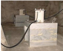
SuperGradiometer installed near Eilat, geophysical laboratory Israel. Sensors and mounting platforms are shown.
