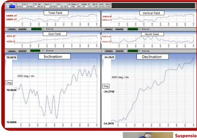
dIdD data output includes; Total Field, Vertical, **North and East** (Z,X,Y) component fields as well as changes to the calculated declination and inclination of the Magnetic Field. The dldD system is designed to measure very subtle changes in the Earth's Field.
