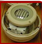
and sensor are located within the sphere and are suspended to ensure the accurate high quality readings and minimimal noise.
