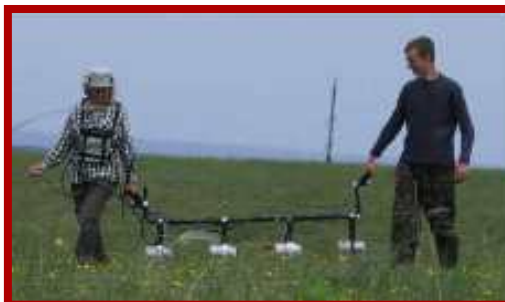
Near surface apparatus for providing increased lateral detection and mapping. Maps and photos courtesy of Dr. Tatiana Smekalova, St. Petersburg State University.
