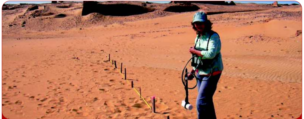
GEM's GSM-19GW magnetometer / gradiometer system (shown above) offers very high sensitivity plus fast sampling rates.
